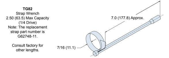
NOTE: Not recommended for composite coupling nuts (use 600-091 or 600-157)
