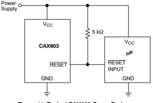
Figure 11. Typical CAX803 Open–Drain Circuit Configuration
