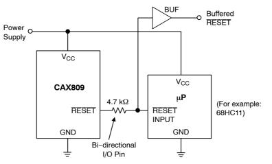
Figure 10. Bi-directional Reset Pin Interfacing
