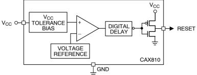
Figure 1. Block Diagrams
