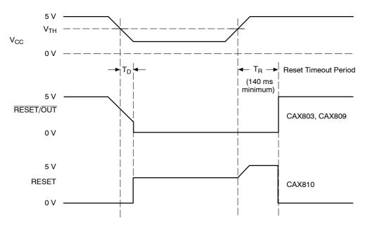
Figure 6. Reset Timing Diagram
