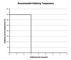
The soldering iron tip temperature should be set at 350°C (+10°C maximum) with the soldering duration not to exceed more than 3 seconds.
