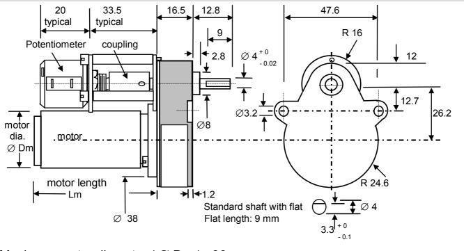
Maximum motor diameter (  $\varnothing$  Dm ) : 36 mm
