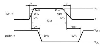
Note 1: Pulse Width 50  $\mu$ s, Duty Cycle 10% Output Impedance 50  $\Omega$ ,  $t_f \le 5$ ns,  $t_f \le 10$  ns
