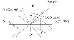
Light (when transmitted )  $Y(\emptyset=0^{\circ})$  $(\theta=90^{\circ})$
