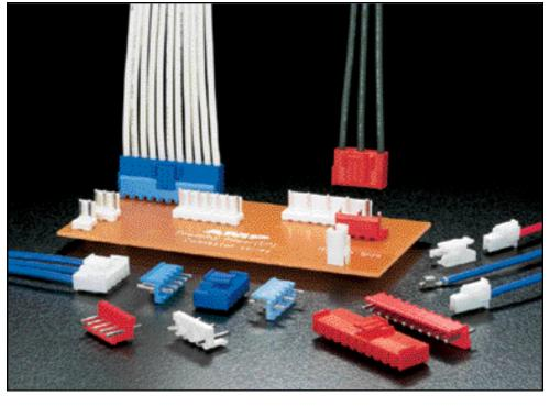
AMP Economy Power (EP) Connectors are designed for secondary power circuit applications. They consist of wire-to-pc board plug housings (for receptacle contacts) and mating post headers. Two contact centerline spacings are available: .156 [3.96] and .312 [7.92].
