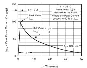
Fig. 3 - Pulse Waveform
