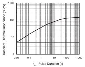
Fig. 6 - Typical Transient Thermal Impedance
