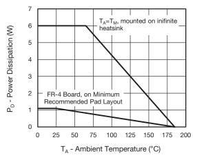
Fig. 5 - Power Dissipation Derating Curve
