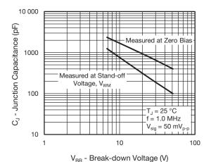
Fig. 4 - Typical Junction Capacitance
