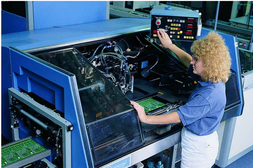
Axial and radial insertion is incorporated into the continuous flow board assembly line.
