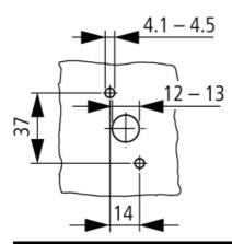
Diameter of drilled hole Door
