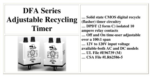
The Amperite DFA series adjustable recycling timers provide a continuously operating off/on cycle as long as power is applied to the input terminals. Two knob operated potentiometers provide user adjustment of both the flash rate and duty cycle. One knob sets the Off time; the other sets the On time. Standard models allow both the Off time and On time to be adjusted over a 100:1 range. Custom timing is available.
