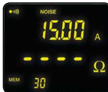
Indicates that the current is greater than 10A
