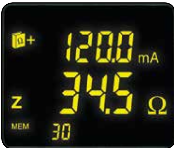
Displays the leakage current and loop impedance at the test frequency
