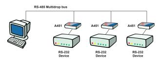
Use two A451 converters to connect RS-232 devices over a long distance using Ethernet cable
