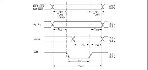
Note: These waveforms are not edge triggered.
