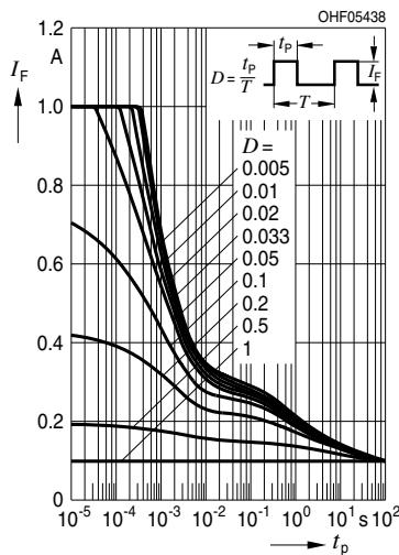
**Permissible Pulse Handling Capability****Zulässige Pulsbelastbarkeit** $I_F = f(t_p)$ ,  $T_A = 85^\circ\text{C}$ , duty cycle D = parameter
