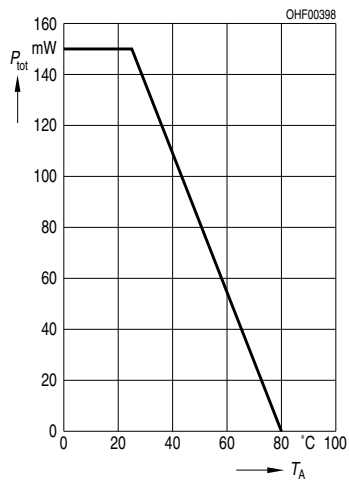
Total Power Dissipation Verlustleistung P_{tot} = f(T_A)
