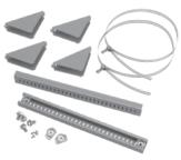
Use to mount CONCEPT<sup>M</sup>, Networking and wall-mount enclosures to poles of various sizes and shapes. Simply attach the plated steel channel bar to the mounting holes at the back of the enclosure and wrap the stainless steel strap around the pole and through the bar. Kit includes two mounting channels, two straps suitable for 3-in. (76-mm) to 12-in. (305-mm) diameter pole and mounting hardware.
