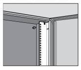
Rack-Mount Angles are a mounting means for 19-in. rack equipment in 24-in. wide enclosures. L-shaped through-hole angles attach to enclosure flange or the adjustable-depth mounting kit. Holes are .281 in. (7 mm) in diameter. Clear plated 14 gauge steel construction. Mounting hardware included.
