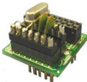
Figure 4-28. Appearance After Mounting Oscillator
