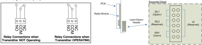
The action of the relay outputs is set by the 'SIL1' Option link setting. A link is made / removed by the small shorting link 'cap' placed over the pin header.
