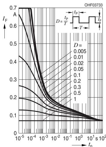
**Permissible Pulse Handling Capability****Zulässige Pulsbelastbarkeit** $I_F = f(t_p)$ ,  $T_A = 85^\circ\text{C}$ , duty cycle D = parameter
