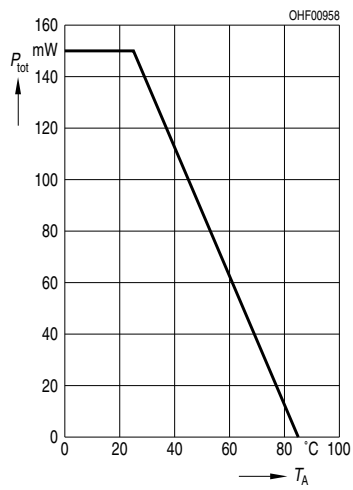
Total Power Dissipation Verlustleistung P_{tot} = f(T_A)
