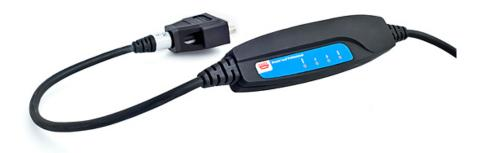
Kvaser Leaf Professional is a one channel, high performance, USB interface for CAN. A versatile and powerful interface that offers easy connection between your PC and CANbus network, it includes Kvaser's patented MagiSync feature for synchronized time-stamping, Galvanic Isolation for protection against voltage spikes, and Auto Transmit for placing messages on the bus at set intervals.
