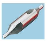
BS 328 Flute geometry Right hand helix Point angle 120° with a 60° Included Countersink Surface treatment Bright Range BS1 (1/8) - BS7 (3/4) Application For producing centre holes in components which require machining between centres.
