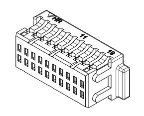
SPECIFICATIONS Current Rating: 1A AC,DC Voltage Rating: 50V AC,DC Temperature Range: -25°C ~ +85°C Contact Resistance: 20mΩ Max. Insulation Resistance: 100MΩ Min. Withstanding Voltage: 500V AC/minute Material: PBT,UL94V-0 Color: Natural(White)
