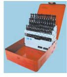
DIN 338 RN/BS 328 Flute geometry Standard helix, right hand spiral Point angle 118° Surface treatment Blue Range 11 piece - 91 piece sets Application General purpose drills in strong retractable cases with each size embossed for ease of identification.
