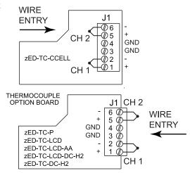
Figure 2.12 Thermocouple Wiring and TC Wire Color Chart
