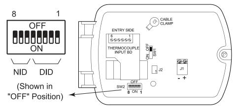
Figure 2.7b Device ID (DID) - 8 Position DIP Switch Setup, zED-DC-H2/zED-LCD-DC-H2
