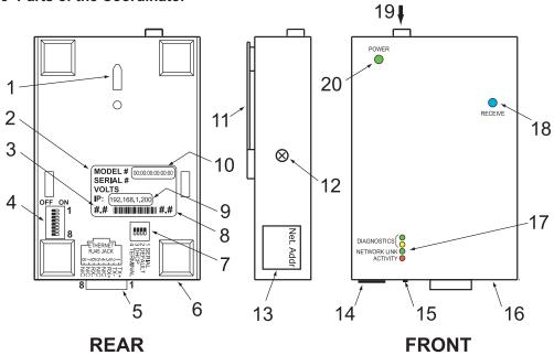
Figure 2.5 Parts of the Coordinator
