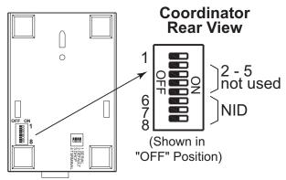
Figure 2.8 Network ID (NID) - 8 Position DIP Switch Setup
