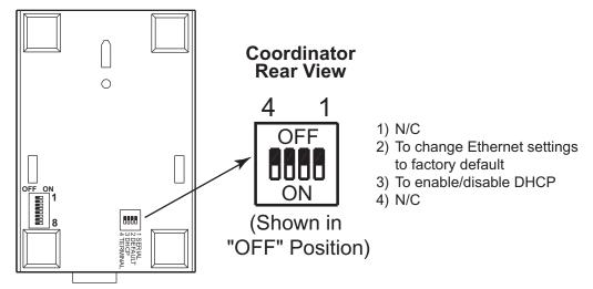
Figure 2.9 Ethernet - 4 Position DIP Switch Setup
