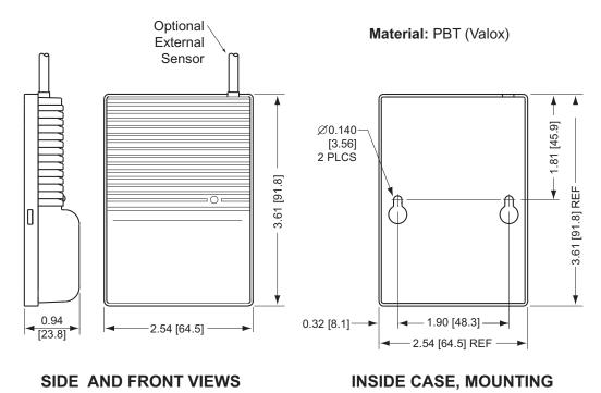
Figure 2.2c Mounting the End Device (zED)
