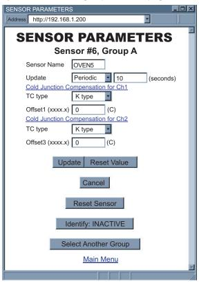
Figure 4.17b Sensor Parameters for Thermocouple Option
