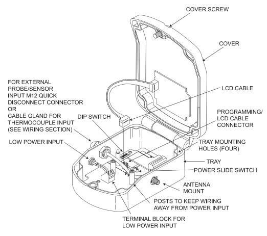
Figure 2.3d Disassembly of the End Device (zED-DC-H2)
