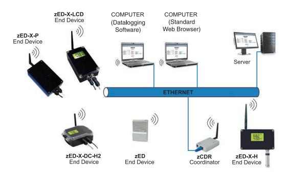
Figure 1.1 zSeries Wireless System on the Ethernet Network
