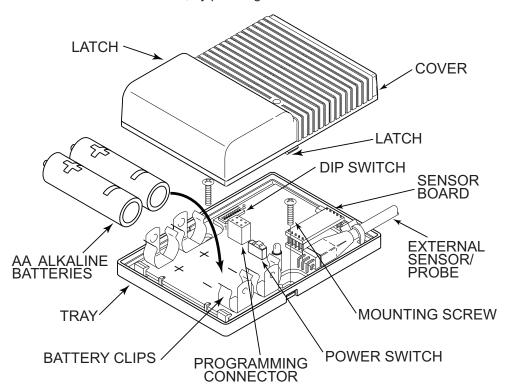
Figure 2.4f Disassembly of the End Device (zED)
