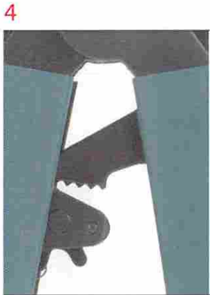
... until the contact is held (1. Ratchet Lever).
