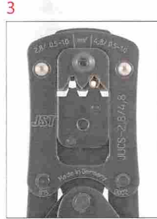
Insert the terminal into the respective profile and close the tool lightly ...
