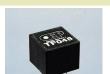
PCB mounting encapsulated 600:600 ⋂ line transformer offering improved performance over the OEP1200 and similar devices. A three part concentrically wound bobbin is utilised to provide improved primary to secondary coupling together with improved frequency response and return loss characteristics.
