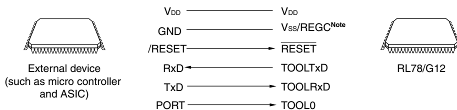
Figure 24-4. Communication with External Device
