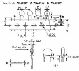
25.4mm pitch/lead spacing 10.0mm taping
