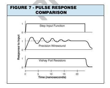
Figure 7 shows the current response to a voltage pulse comparing a fast Bulk Metal® Foil resistor to a slower wirewound resistor. Here a pulse width of one nanosecond would have been completely missed by the wirewound resistor while the Vishay Foil resistor achieves full replication in the time allotted.
