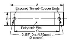
Grounds made with ordinary wire (e.g., #18 copper wire) will have high impedance at RF frequencies, and can actually act as an antenna, thereby increasing radiated emission levels. Braided ground straps are costly and inconvenient because their ends generally require tinning or hole punching by the user, and they must often be insulated to avoid shorting problems in tight quarters.
