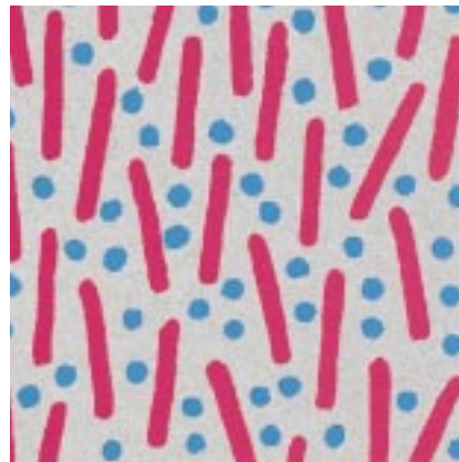
Illustration 200.9: The structure of iglidur®: base polymer, fillers and solid lubricants
