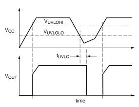
Figure 3. Definition of Undervoltage Lockout
