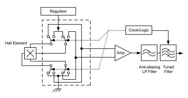
Figure 6. Chopper Stabilization Technique
