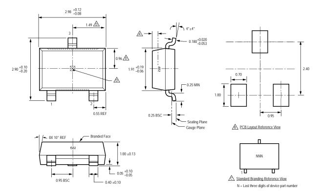
For Reference Only; not for tooling use (reference DWG-2840) Dimensions in millimeters
