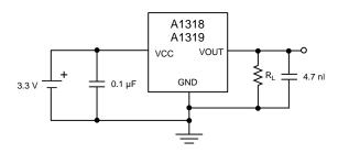
Figure 5. Typical Application Circuit
