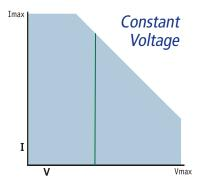
Constant voltage mode is used for load testing of constant current power supplies. The unit operates as a high power shunt regulator.
