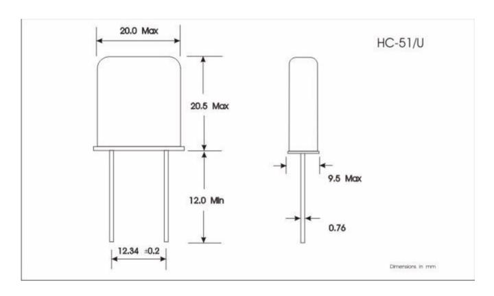
Holder Style Mode Adjustment Tolerance Temperature Stability Operating Temp. Range Load Capacitance Marking HC51U Fundamental ± 50PPM at 25°C ± 100 PPM -10°C to +60°C 30 pF Mark AELX001L\FREQ+WWYY
