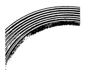
Copper tubing to BS 2871 : Part 2 with dimensions generally to table 4
