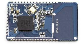
nRF51822-QFAA is an ultra-low power 2.4 GHz wireless System on Chip (SoC) integrating the
