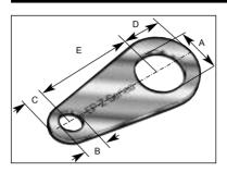
**EP-Z Series** Earth Tags are used to provide an earthbond connection for an entry component.
