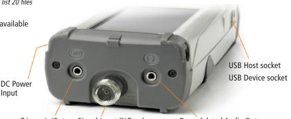
Trigger In/Out Signal Input (N Type)
