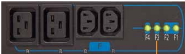
LEDs represent each outlet
