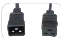
010-9342: C20 Male to C19 20A 8-foot, 12 AWG/3-wire
