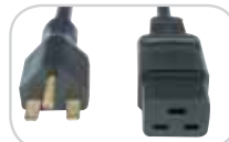
010-9336: 6-15P to C19 125V, 15A straight blade 8-foot, 14 AWG/3-wire
