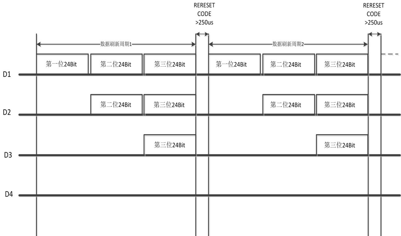
Note: D1 is the data from MCU, and D2, D3, D4 are from Cascade Circuits.
