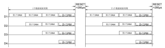
Note: The data of D1 is send by MCU, and D2, D3, D4 through pixel internal reshaping amplification to transmit.
