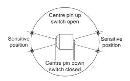
Contact Form/Style: Switch types CM1800 may have a normally open or closed contact depending on the positioning of the switch. These switches have a change in sensitivity depending on the switch position.
