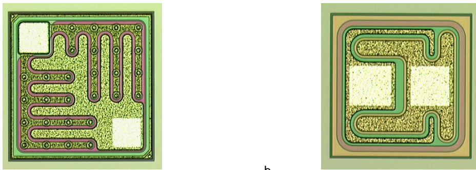
Fig 1. The die layout of a mesh-emitter transistor (a.) clearly shows the characteristic finger structure. Compared to the typical die layout of a conventional transistor (b.), a mesh-emitter transistor's finger structure and base contact holes provide a much larger active area.
