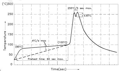
1.Recommend pre-heat temperature of 105°C or less (as measured with a thermocouple attached to the LED pins) prior to immersion in the solder wave with a maximum solder bath temperature of 260°C
