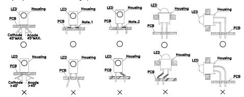
"() " Correct mounting method "imes" Incorrect mounting method
