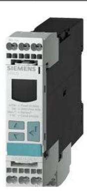
DIGITAL MONITORING RELAY VOLTAGE MONITORING, 22.5MM FROM 17 TO 275V AC/DC OVERSHOOT AND UNDERSHOOT INTERNAL POWER SUPPLY DC AND AC 50 TO 60 HZ SPIKE DELAY 0.1 TO 20S HYSTERESIS 0.1 TO 150V 1 CHANGEOVER CONTACT W. OR W/O ERROR LOG SCREW TERMINAL REPLACEMENT PRODUCT F. 3UG3534, 3UG3535
