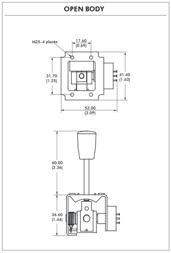
NOTE: The dimensions shown are for a generic two axes 4000 Series open body with the E type handle, and a generic two axes 4000 Series closed body also with the two axes E type handle. For specific dimensions of this or any other configuration please refer to Apem.
