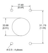
The joystick mounts from beneath the panel and the boot is trapped between the joystick and the panel. No bezel is necessary for this installation, since the panel acts as the bezel. The frame has M2.5 tapped holes and as such M2.5 machine screws are recommended for this mounting.
